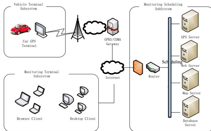
**Fig. 2** Physical Structure of Shuttle Bus Monitoring Scheduling Subsystem
