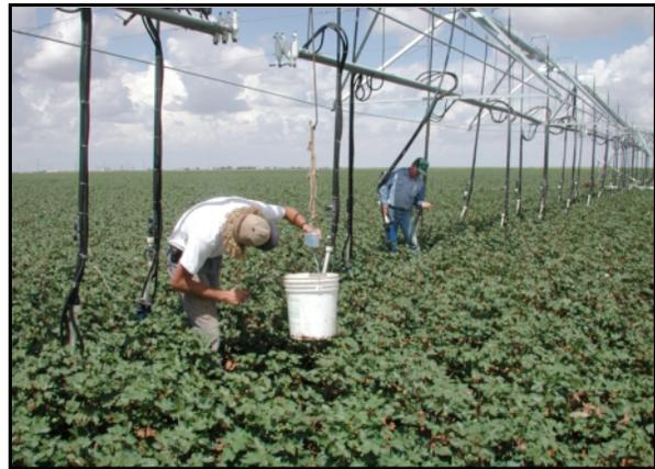
Figure 1. Evaluation of the hydraulic performance of a VR irrigation system, TAES, Helms Farm, 2001.
