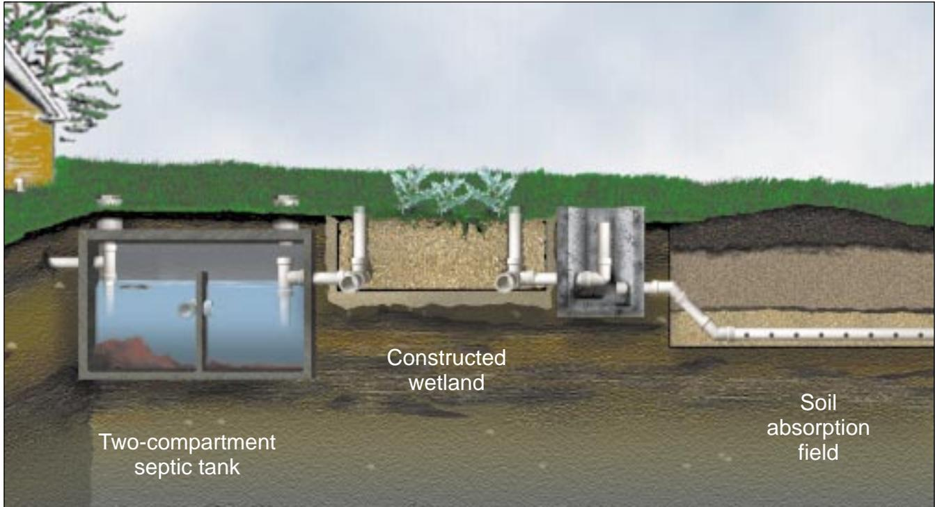
Figure 1: A constructed wetland system.
