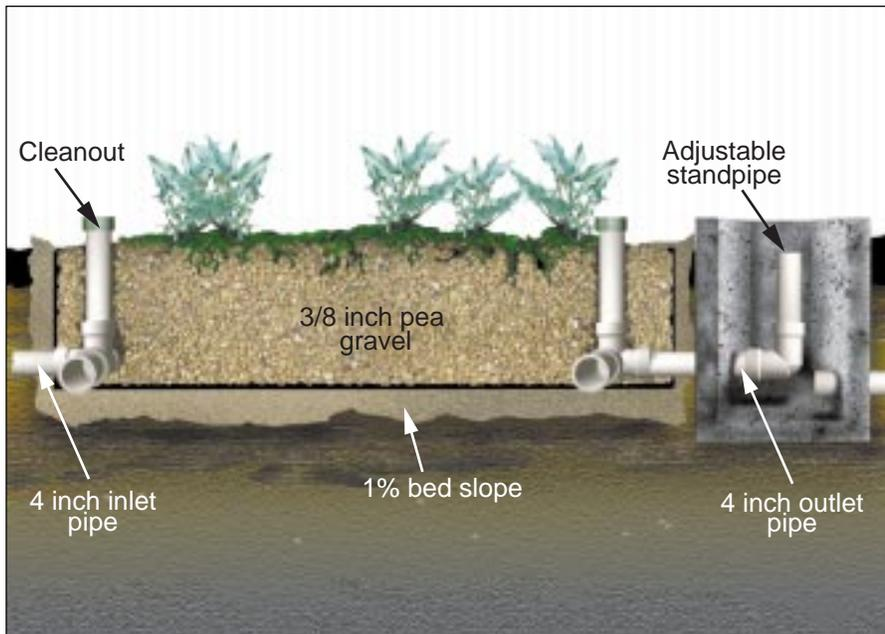
**Figure 2:** A constructed wetland is a bed of graded stone where water flows beneath the surface and plants grow on top.
