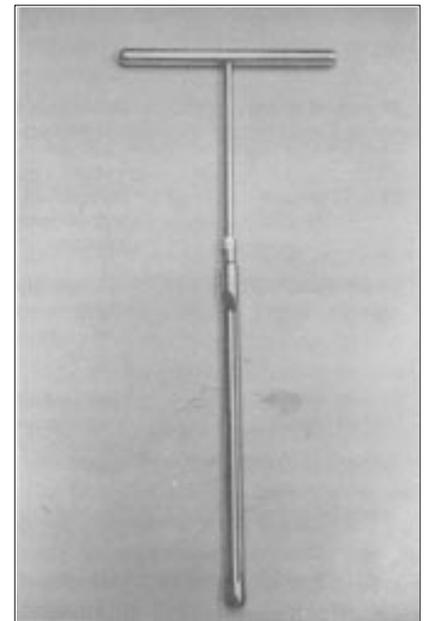
Figure 1: Soil Probe
