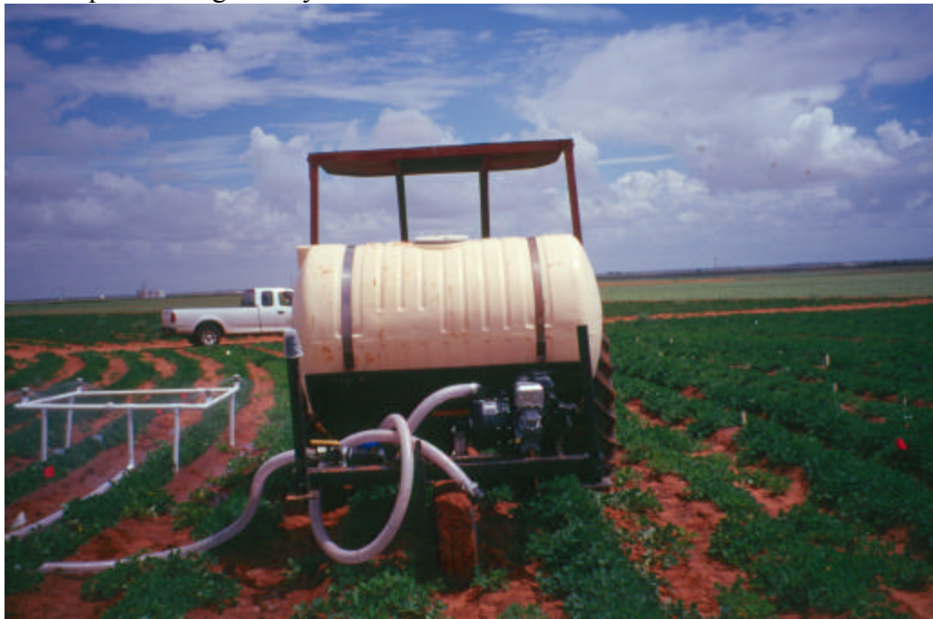
Fig. 2. Small plot chemigation system
